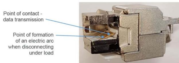
*Section of an RJ45 module in the region of the contact springs*
