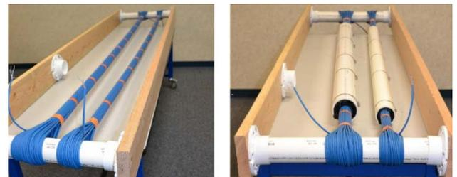
In order to simplify installation practice as much as possible, the standard recommends a maximum of 37 cables per bundle throughout. If the cable properties, the installation environment and the effective PoE landscape are included in the planning process, however, other bundle sizes are also acceptable.
