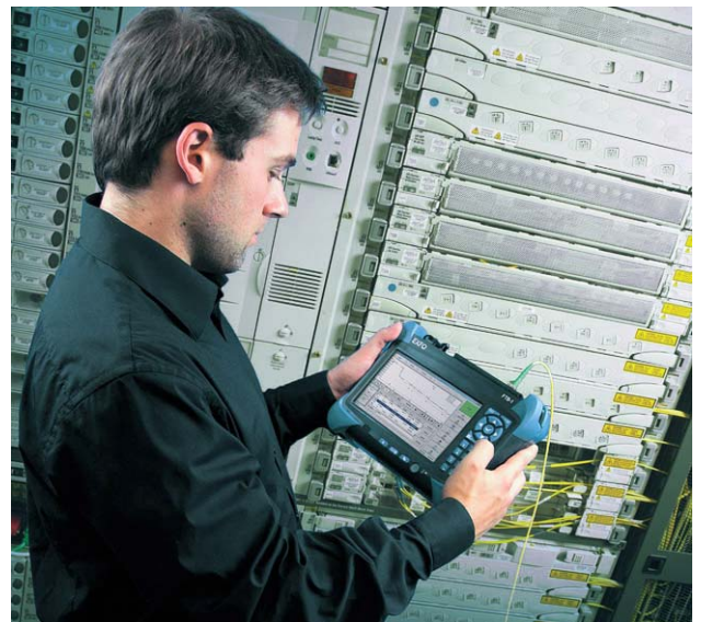
Image 1: OTDR testing a section of FO cabling. © EXFO/Opternus
